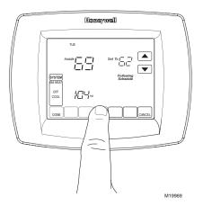
**3.** The User Setup Number is displayed in the lower-left screen. It is a four-digit code beginning with zero. Current setting is displayed in lower-right screen.
